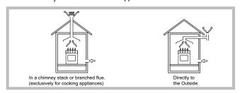
The room must also allow proper air circulation, as air is needed for combustion to occur normally. The flow of air must not be less than 2 m<sup>3</sup>/h per kW of installed power.
